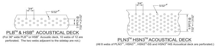
Figure 2 - Fully Perforated Deck Patterns
